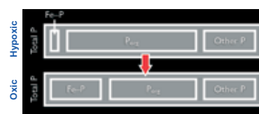
Figure 2. When oxygen conditions change from hypoxic to oxic organic phosphorus is remineralised and becomes iron-bound. The iron-bound pool will be released from the sediments to the water if sediments become hypoxic again (P-bomb).
